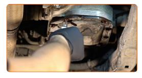
10 Remove the transmission fluid pan.
