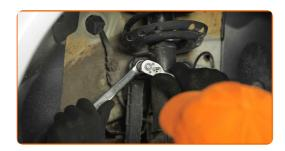
Unscrew the fastener connecting the stabilizer link to the stabilizer bar. Use a combination spanner #18. Use Torx T30. Use a ratchet wrench.
