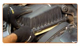
6 Remove the filter element from the filter housing.
