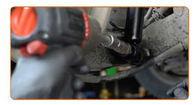
9 Remove the fastening bolt.
