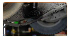
10 Remove the mounting from under the rear axle beam.
