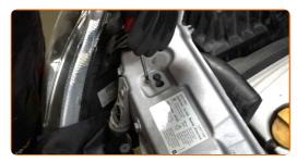
Remove the air distribution housing assembly.
