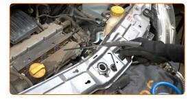
Detach the connector from the ignition coil. Use a flat screwdriver.
