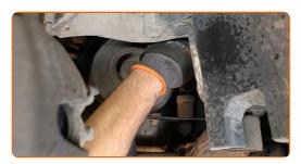
Return the tensioner pulley to its initial position. Use a combination spanner #19.
