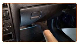
Screw the glove box fastening screws. Use Torx T20.
