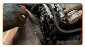
Unscrew the filter housing cap together with the old filter element. Use a drive socket #36. Use a ratchet wrench.
