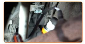
Attach the oxygen sensor connector.
