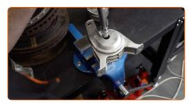
Remove the bracket with the engine mount from the vice.
