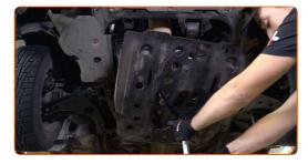
Support the engine skid plate. Use a hydraulic transmission jack.
