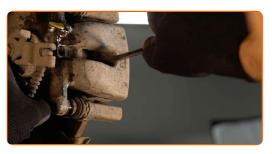
Remove the brake caliper. Use a crowbar.
