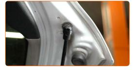
13 Install the new boot lid gas strut.
