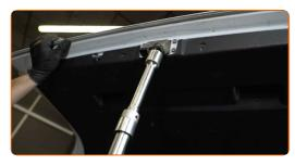
Release the circlip connecting the gas strut to the boot lid. Use a flat screwdriver.
