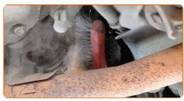
Detach the oxygen sensor connector.
