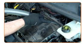
Insert a new filter element into the filter housing.
