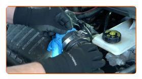
6 Detach the connector from the MAF sensor.
