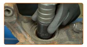
Press the outer bearing race together with the bearing's internals and the ABS sensor bracket out of the steering knuckle. Use a bush and bearing driver set and a hydraulic press.
