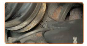
Detach the ABS sensor wiring.
