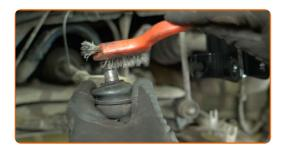
Clean the steering knuckle mounting seat on the suspension strut. Use a wire brush. Use an all-purpose cleaning spray.
