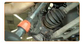
67 Secure the brake hose to the suspension strut.
