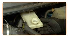
79 Tighten the brake fluid reservoir cap.
