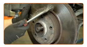
Unscrew the brake disc screw. Use a T40 Torx bit. Use a ratchet wrench.
