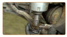
Disconnect the tie rod end from the steering knuckle. Use a ball joint separator.
