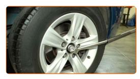
Loosen the wheel fasteners. Use a 19 mm wheel impact socket. Use a tommy bar.
