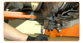
Replacement: wheel bearing – VAUXHALL Vivaro Platform / Chassis (X83). AUTODOC recommends:
