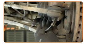
Unscrew the axle nut. Use a 32 mm socket. Use a ratchet wrench.
