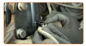
Secure the ABS sensor wiring.
