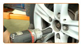
Lower the car and tighten the wheel fasteners in a criss-cross pattern. Use a 19 mm wheel impact socket. Use a torque wrench. Tightening torque: 142 N·m.
