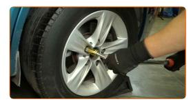
75 Tighten the axle nut. Use a 32 mm socket. Use a torque wrench. Tightening torque: 280 N·m.
