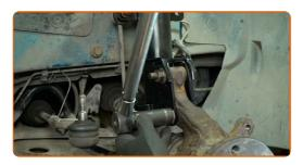
Tighten the fasteners that connect the ball joint to the control arm. Use an 18 mm combination spanner. Use a 19 mm socket. Use a torque wrench. Tightening torque: 85 N·m.
