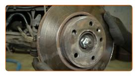
62 Install the brake disc screw.
