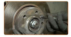
Tighten the brake disc screw. Use a T40 Torx bit. Use a torque wrench. Tightening torque: 14 N·m.
