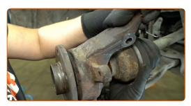
Attach the steering knuckle to the suspension strut.
