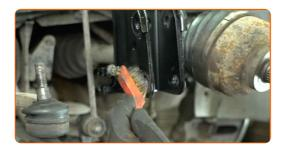
Clean the splines of the CV joint. Use a wire brush. Use an all-purpose cleaning spray.
