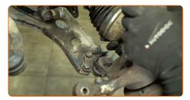
Remove the steering knuckle together with the wheel hub.
