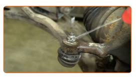
Unscrew the nut connecting the tie rod end to the steering knuckle. Use a 16 mm socket. Use a ratchet wrench.
