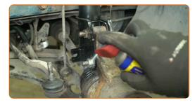
Unscrew the fasteners that connect the suspension strut to the steering knuckle. Use a 21 mm combination spanner. Use a 21 mm socket. Use a ratchet wrench.
