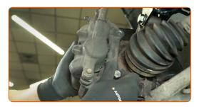
Tighten the fasteners of the brake caliper bracket. Use an 18 mm socket. Use a torque wrench. Tightening torque: 100 N·m.
