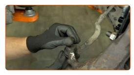
Tighten the nut connecting the tie rod end to the steering knuckle. Use a 16 mm socket. Use a torque wrench. Tightening torque: 37 N·m.
