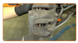
Detach the brake hose from the suspension strut.
