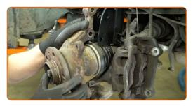
Detach the CV axle from the steering knuckle.
