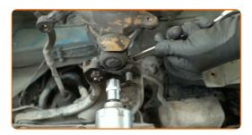
Clean the fasteners that connect the suspension strut to the steering knuckle. Use a wire brush. Use WD-40 spray.
