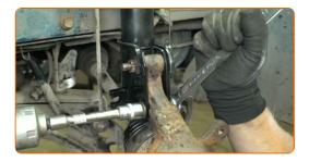
Remove the fastening bolts. Use a pin punch. Use a hammer.
