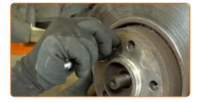
Remove the brake disc.
