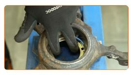
Replacement: wheel bearing – VAUXHALL Vivaro Platform / Chassis (X83). Tip:
