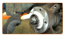
61 Install the brake disc.
