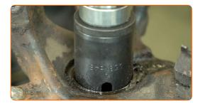
Press the hub out of the inner race of the bearing. Use a bush and bearing driver set. Use a bearing separator and a hydraulic press.
