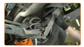
Clean the shock absorber mounting seats. Use a wire brush. Use an all-purpose cleaning spray.
