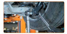
Tighten the upper fastener of the shock absorber. Use a 21 mm combination spanner. Use a 21 mm socket. Use a torque wrench. Tightening torque: 180 N·m.
