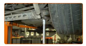
Unscrew the lower fastener of the shock absorber and remove the stop plate. Use a 21 mm combination spanner. Use a 21 mm socket. Use a ratchet wrench.
