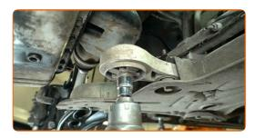
Unscrew the fastener that connects the engine mount to the subframe. Use an 18 mm socket. Use a ratchet wrench.
