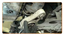
Replacement: engine mounts – VAUXHALL Vivaro Platform / Chassis (X83).
