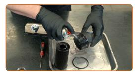
Install a new O-ring on the oil filter cap. Install a new filter element into the oil filter cap.
