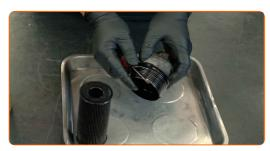
Clean the oil filter cap. Use an all-purpose cleaning spray.
