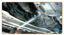
Unscrew the filter cap together with the old filter element. Use a 27 mm socket. Use a ratchet wrench.
