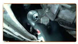
Remove the filter element from the filter cap. Remove the old O-ring of the oil filter cap. Use a slotted screwdriver.
