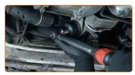
Clean the area of the oil pan drain hole. Use an all-purpose cleaning spray.
