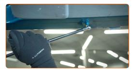
15 Install the new left gas strut on the rear door.
