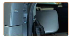
Snap on the retaining clip connecting the left gas strut to the car body.
