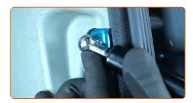
Snap on the retaining clip connecting the right gas strut to the rear door.
