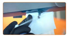
Apply grease to the ball sockets of the new gas struts if they are not sold pregreased. Use multipurpose grease.
