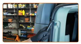
Clean the mounting seats of the left gas strut. Use an all-purpose cleaning spray.
