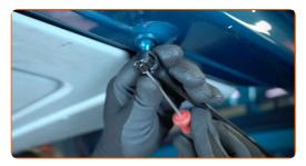
Release the retaining clip connecting the right gas strut to the vehicle body. Use a slotted screwdriver.
