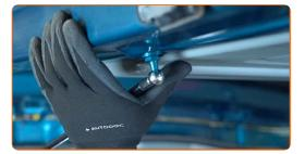
Snap on the retaining clip connecting the left gas strut to the rear door.
