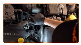
Return the coolant pipe to its initial position and fasten it.
