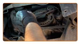
Place the V-ribbed belt on the tensioner pulley.
