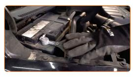
Screw in the fastener of the wiper cowl grille located on the left side. Use Torx T25.
