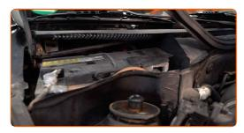
Remove the wiper cowl grille located on the left side.
