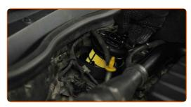
Tighten the fasteners of the fuel filter housing cover.
