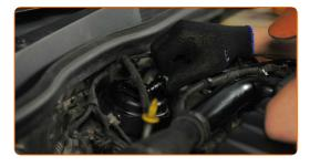
17 Attach the fuel pressure sensor connector.
