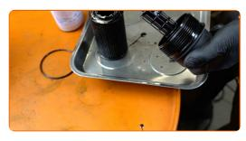
Clean the oil filter housing cap. Use all-purpose cleaning spray.
