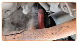
Detach the oxygen sensor connector.
