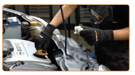
33 Tighten the oil filler cap.
