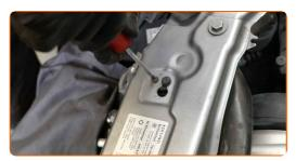
Remove the fender protection cover.
