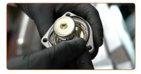
Install a new thermostat housing.
