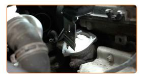
Remove the microfibre cloth from the mounting seat of the thermostat housing.
