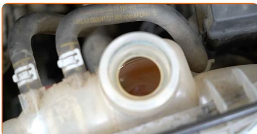
**46** Install the coolant reservoir cap.
