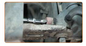
Drain the coolant from the engine.
