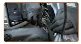
Secure the coolant hose clamp. Use clic-R collar pliers.
