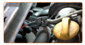
Detach the coolant hose. Use a flat screwdriver.
