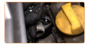
Remove the thermostat housing.
