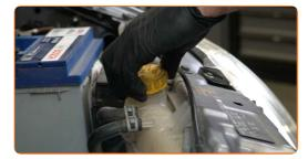
Pour coolant in the coolant reservoir.
