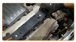
Tighten the ignition coil bolts. Use Torx T30. Use a torque wrench. Tighten it to 7 nm torque.
