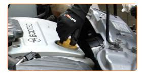
Tighten the oil filler cap.
