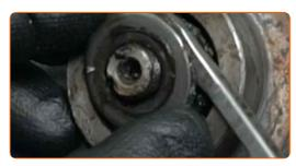
Remove the wheel hub bearing. Use a crowbar.
