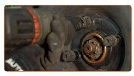
Lower the car and working in a cross order, tighten the wheel bolts. Use wheel impact socket #17. Use a torque wrench. Tighten it to 110 Nm torque.
