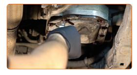
10 Remove the transmission fluid pan.
