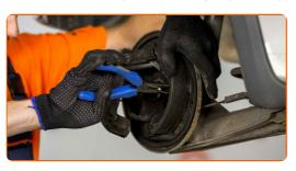
15 Remove the brake pads.
