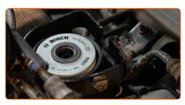
Put the fuel filter cap back on.
