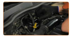
17 Attach the fuel pressure sensor connector.
