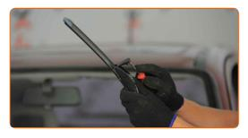
Remove the blade from the wiper arm.
