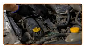
Take out the ignition coil from the spark plug well. Use a flat screwdriver.
