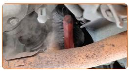
Detach the oxygen sensor connector.
