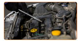
Replacement: spark plugs – VAUXHALL Omega (B) Estate (V94). Tip from AUTODOC:
