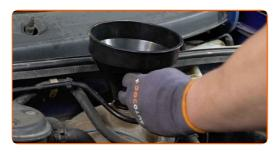
Pour coolant in the coolant reservoir.
