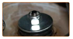
28 Tighten the lower fastener of the shock absorber. Use a drive socket #17. Use a torque wrench. Tighten it to 65 Nm torque.
