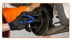
15 Remove the brake pads.
