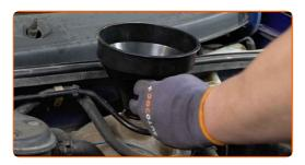
Pour coolant in the coolant reservoir.
