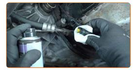
Install the new retaining spring of the crankshaft position sensor.
