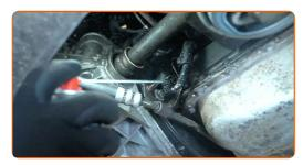
Detach the connector of the crankshaft position sensor. Use a mounting lever.
