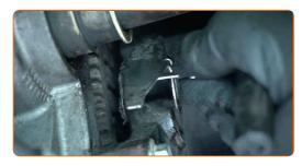
Clean the mounting seat of the crankshaft position sensor. Use a wire brush. Use an all-purpose cleaning spray.
