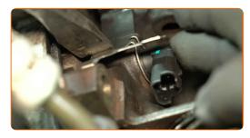
Attach the connector of the crankshaft position sensor.
