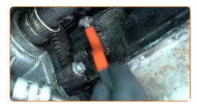
Treat the connector of the crankshaft position sensor. Use an electronic spray.
