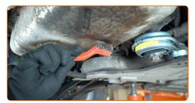
Unscrew the drain plug. Use an 8 mm square head drain plug socket. Use a ratchet wrench.
