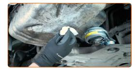
Screw in the drain plug and tighten it. Use an 8 mm square head drain plug socket. Use a torque wrench. Tightening torque: 20 N·m.
