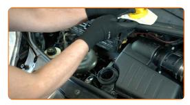
Pour oil into the engine through the filler neck. Required amount of oil: 8 L.
