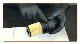
Install the oil filter cap and screw it in. Use a 27 mm socket. Use a torque wrench. Tightening torque: 25 N·m.
