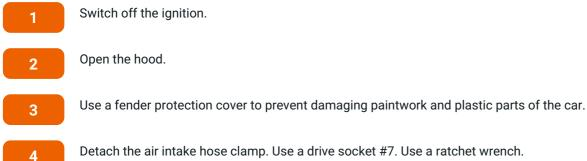
Detach the air intake hose clamp. Use a drive socket #7. Use a ratchet wrench.
