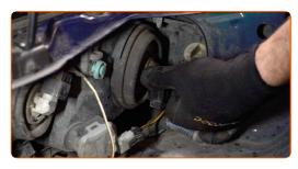
Remove the old bulb. Use a flat screwdriver.
