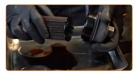
Remove the oil filter cover O-ring. Use a flat screwdriver.
