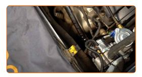
Remove the oil filler cap. Insert the funnel.
