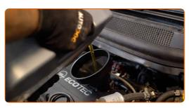
Replacement: engine oil and filter – VAUXHALL Meriva Mk II (B) (S10). AUTODOC recommends:
