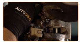
Tighten the brake hose fastener. Use a drive socket #11. Use a torque wrench. Tighten it to 40 Nm torque.
