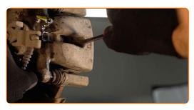
Remove the brake caliper. Use a crowbar.
